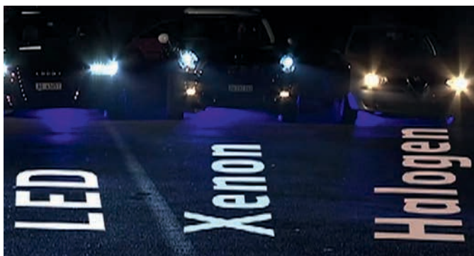
Figure 8. Different color temperatures of LED, HID/Xenon and Halogen headlights when compared side by side (examples).
