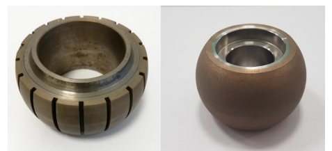
Figure 12. The highly complex ZEISS ClearView lens design is incorporated into the lens molds using CNC generators using grinding tools containing millions of diamond particles.
