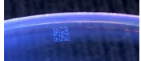
Figure 14. Data Matrix Code (DMC) at the very edge of the final uncut lens.
