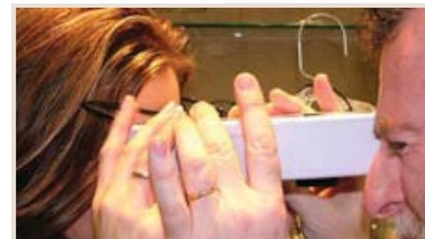
1. Set distance wheel to infinity ( $\infty$ ) for far PD or the correct near distance 35cm= $\sim$ 14 inches, 40cm= $\sim$ 16 inches, 45cm= $\sim$ 18 inches
