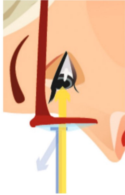
FIG. 20 FRONTSIDE: With a STANDARD AR, visible light passes through the lens as intended while the material absorbs most of the UV rays. Some UV is reflected from the AR-coated lens surface.
